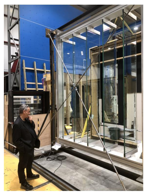
on avenue bernanos, the facades will be renovated by installing external insulation by creating a ventilated surface. this second envelope made of silkscreened glass louvers acts as a solar shading device. atex certification was obtained in july 2024 (cstb) entreprise kingspan
